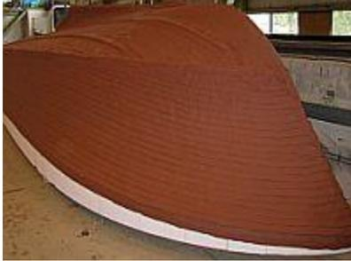
Huntsman Advanced Materials has a new solution for making plugs and moulds for the marine sector whilst offering cost savings and time intensive production processes through its range of RenPaste epoxy seamless modelling pastes.
