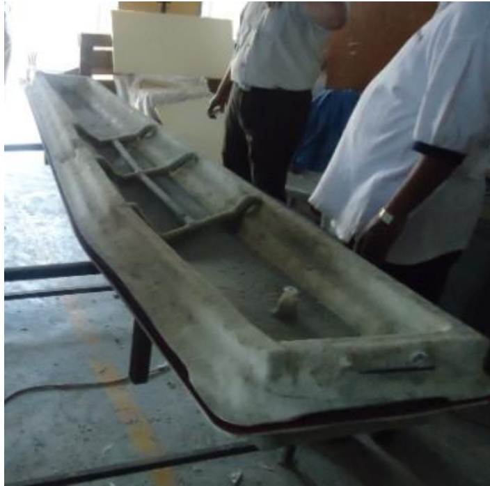
Mold Closure – Vacuum Application
